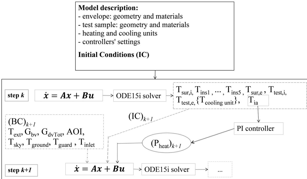
Fig. 1. Structure of the Matlab code. The term {Tcooling unit} refers to the temperature nodes in the cooling unit (metallic parts and water layer).
