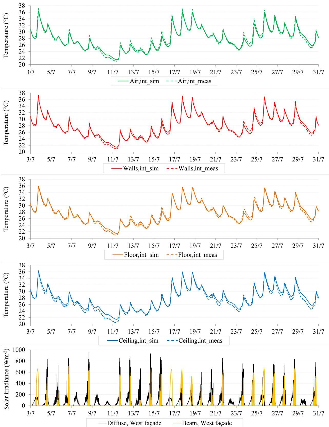
**Fig. 4.** Top four graphs: simulated (sim) and measured (meas) average temperatures of the internal air, the (North, East and South) walls' internal surfaces, the floor and the ceiling. Bottom: diffuse (sky-diffused + ground-reflected) and beam solar radiation on the West façade.
