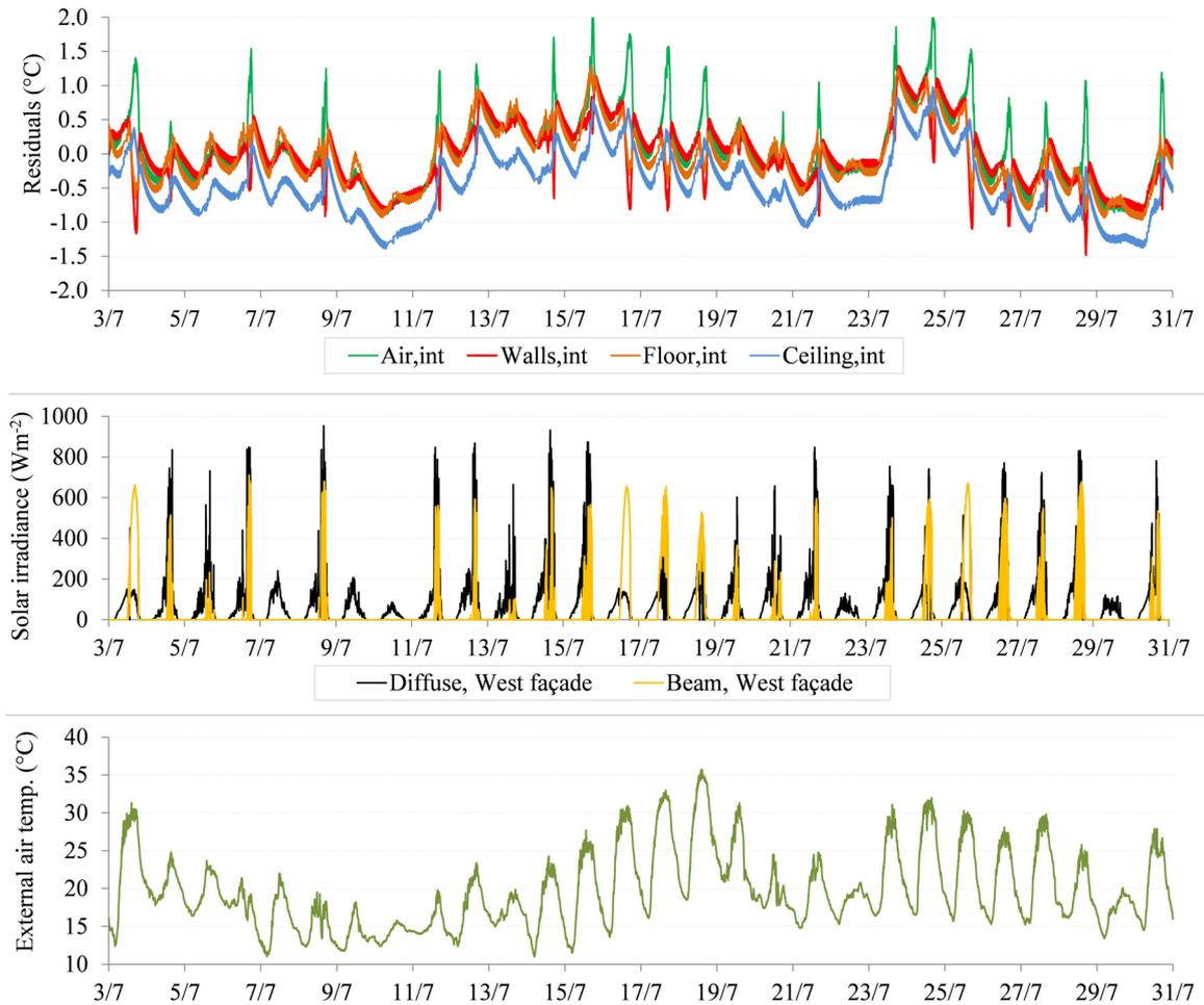
Fig. 5. Top: profiles of residuals (calculated as measured minus predicted); centre: total diffuse (including sky-diffused and ground-reflected radiation) and beam solar radiation on a vertical surface exposed to west; bottom: external air temperature.
