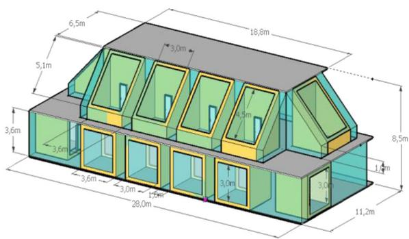
Fig. 2. BESTLab Platform: external view (with indication of the test cell used in the present work) and scheme. Sources: Bontemps et al. Bontemps et al. (2015) and EDF (2016).
