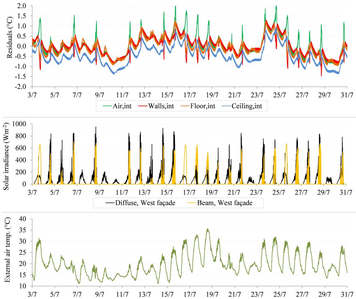
**Fig. 5.** Top: profiles of residuals (calculated as measured minus predicted); centre: total diffuse (including sky-diffused and ground-reflected radiation) and beam solar radiation on a vertical surface exposed to west; bottom: external air temperature.
