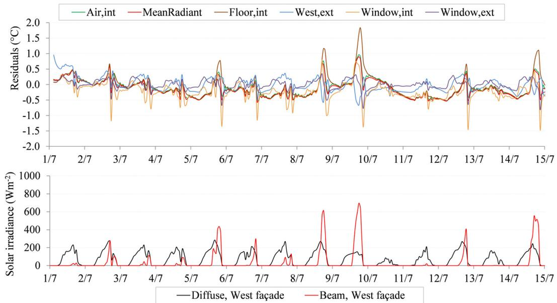
Fig. 6. Top: temperature residuals of the intermodel comparison: internal air temperature, mean radiant temperature, floor surface temperature, temperature of the external surface of the West wall, temperatures of the internal and external panes of the window component. Bottom: total diffuse (including sky-diffuse and ground-reflected radiation) and beam solar radiation on a vertical surface exposed to west.
